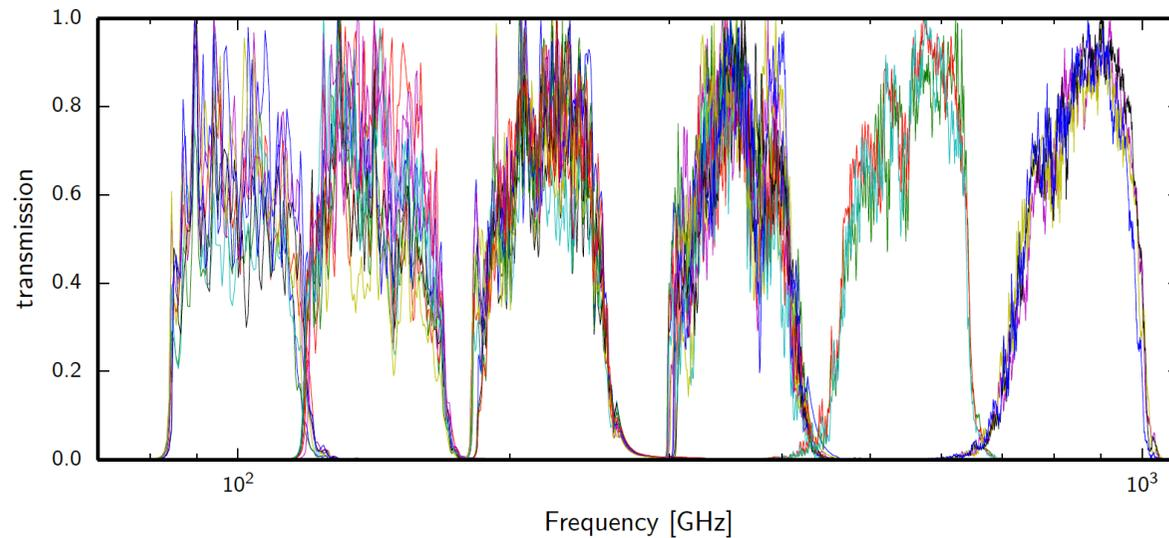
CO transition line 1- $\rightarrow$  0 falls at the edge of the 100 Hz filters so the CO components has very different amplitude from detector to detector
