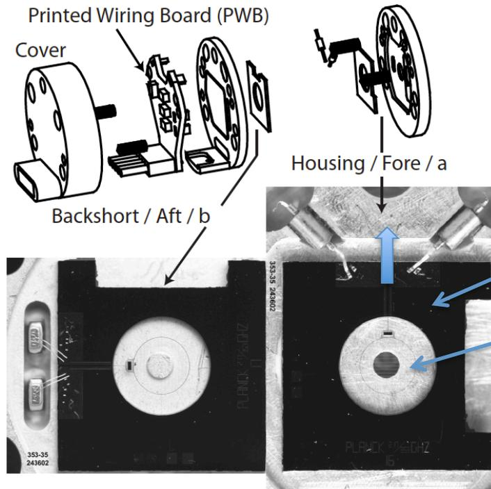
Thermal modeling is important. Long time constants come from the links between the wafer and the detector housing
