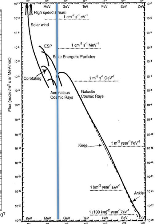
Cut off due to material around the detectors at  $\sim 50$  MeV
