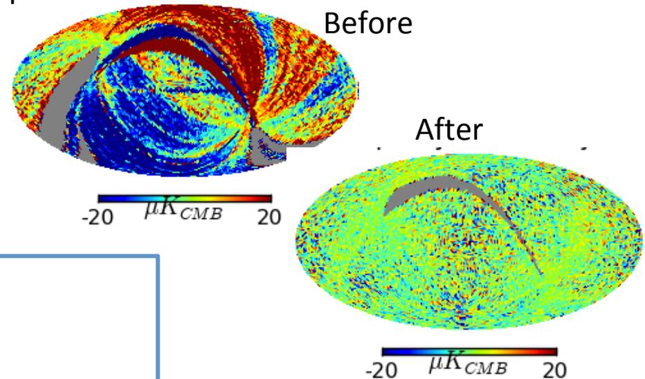
ADC is the limiting systematic effect in Planck for polarization measurement
