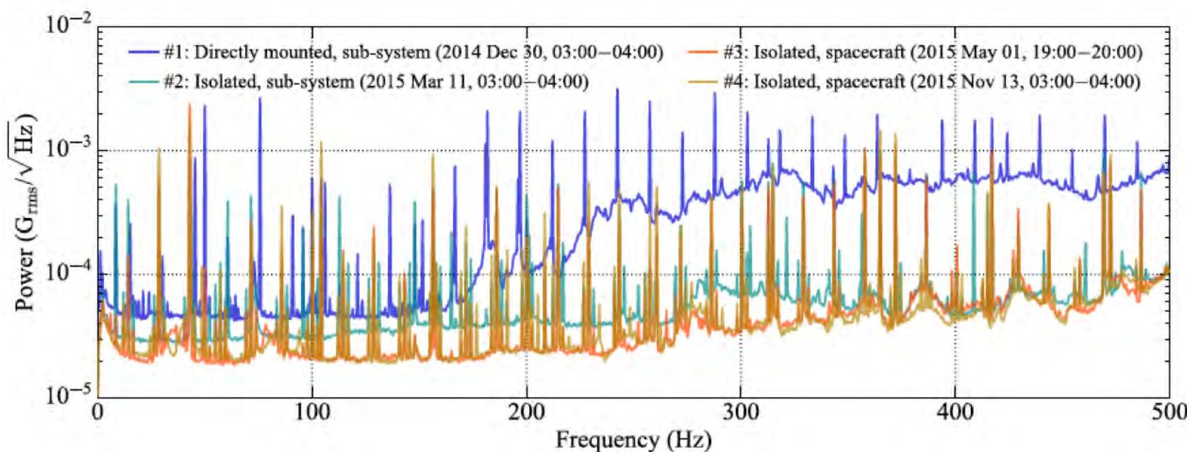
Power spectrum of microphonic vibration of Hitomi
