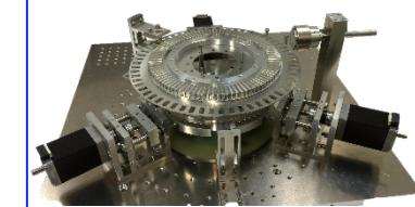
Continuously-rotating half wave plate (HWPs) for LFT and HFT
