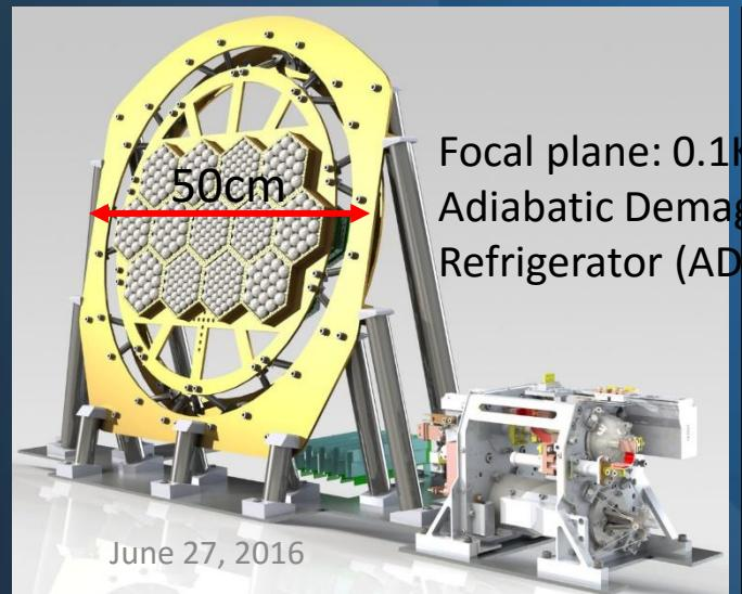
2622 TES bolometers cover 15 bands in the frequency range of 40 to 400 GHz.
