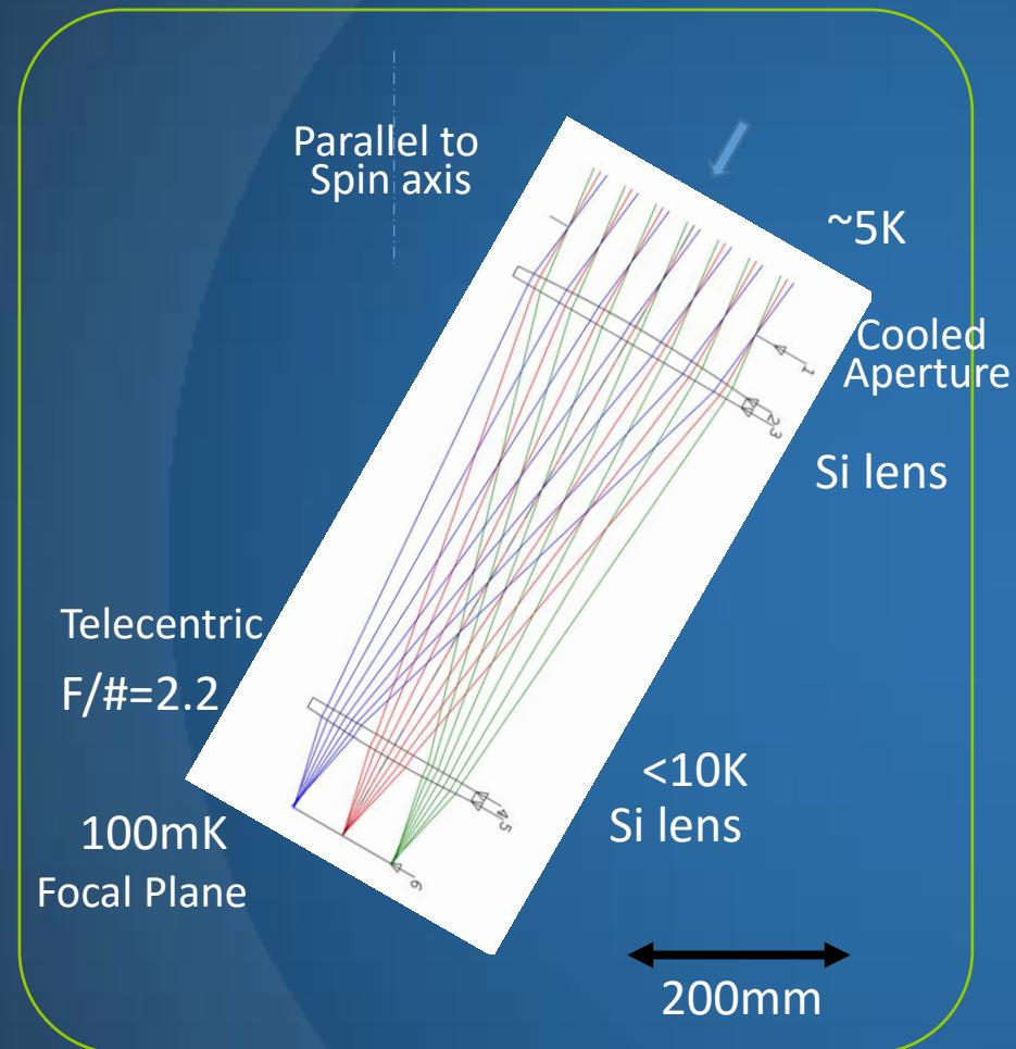
High Frequency (280-402GHz) telescope
